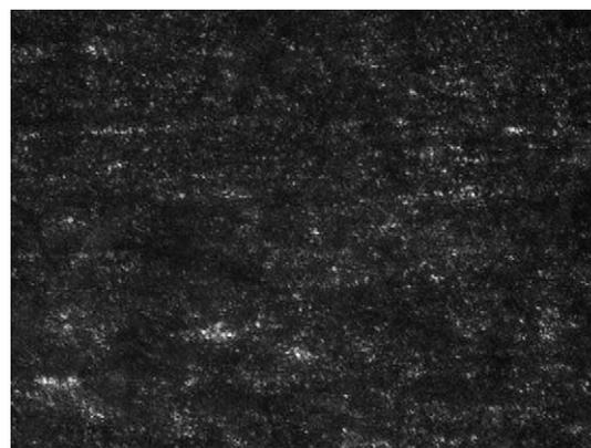
Fig. 3. Micrograph showing copper (UNS C10200) covered with a mat of bacterial cells, the coupon had been left for 90 min at room temperature. Episcopic differential interference contrast (EDIC) image showing a dense mat of bacteria on the surface of the copper coupon. Mag.  $\times 500$ .
